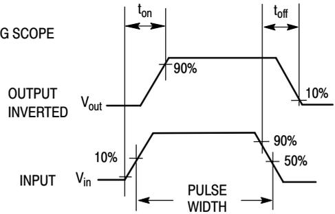
Figure 2. Switching Waveforms
