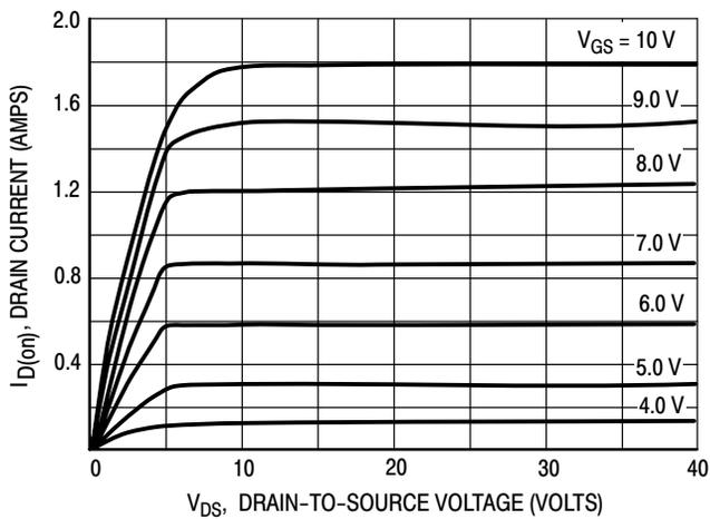
Figure 5. Output Characteristics
