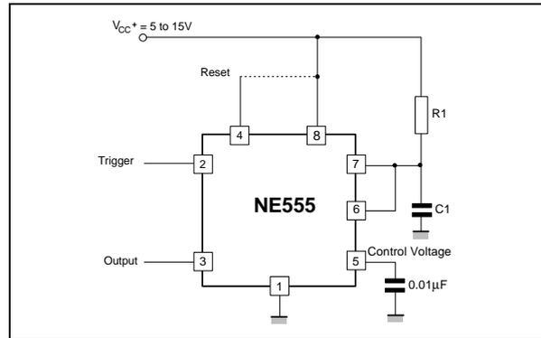
The circuit triggers on a negative-going input signal when the level reaches 1/3 V<sub>CC</sub>. Once triggered, the circuit remains in this state until the set time has elapsed, even if it is triggered again during this interval. The duration of the output HIGH state is given by  $t = 1.1 R_1 C_1$  and is easily determined by figure 12.
