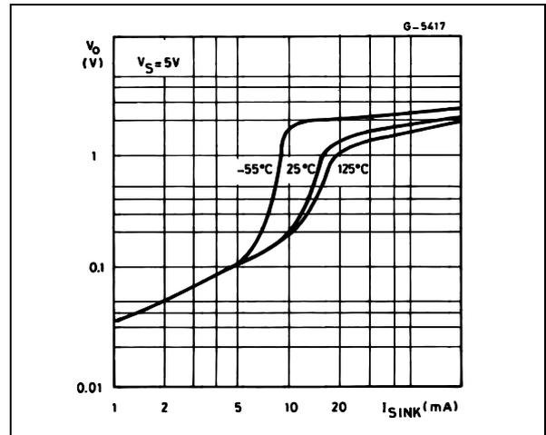
Figure 5 : Low Output Voltage versus Output Sink Current
