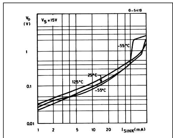
**Figure 7 :** High Output Voltage Drop versus Output
