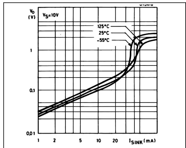
Figure 6 : Low Output Voltage versus Output Sink Current
