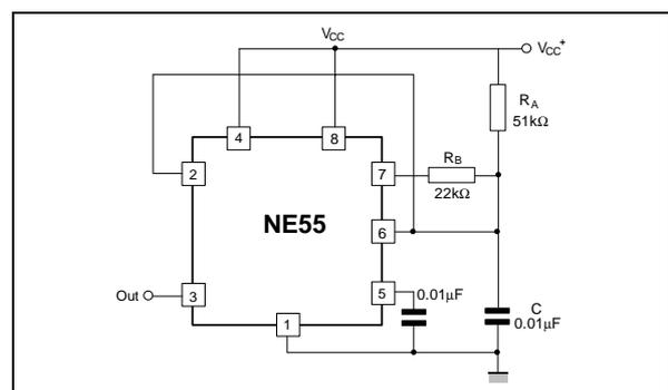
Note that this circuit will not oscillate if RB is greater than 1/2 RA because the junction of RA and RB cannot bring pin 2 down to 1/3 VCC and trigger the lower comparator.
